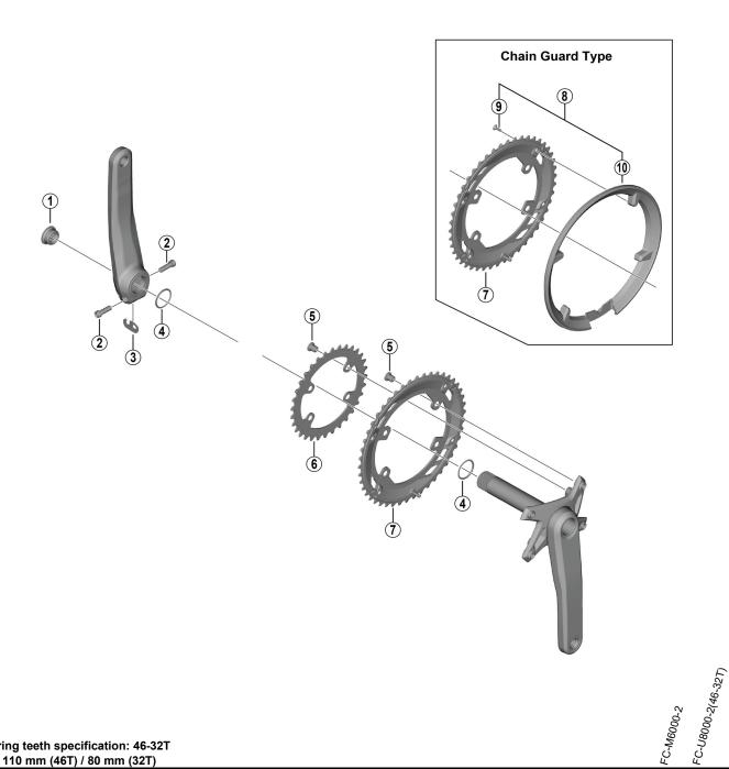
• Chainring teeth specification: 46-32T • P.C.D. 110 mm (46T) / 80 mm (32T)
